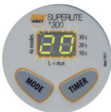
Timer flashes low battery 5-10% charge!
